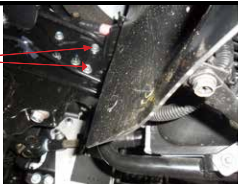
Drivers side rear of condenser mount pictured
