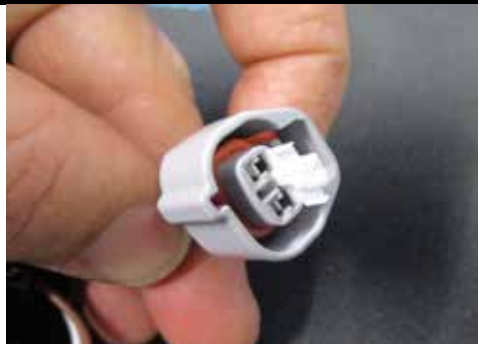
Close up of terminal showing locking tab area
