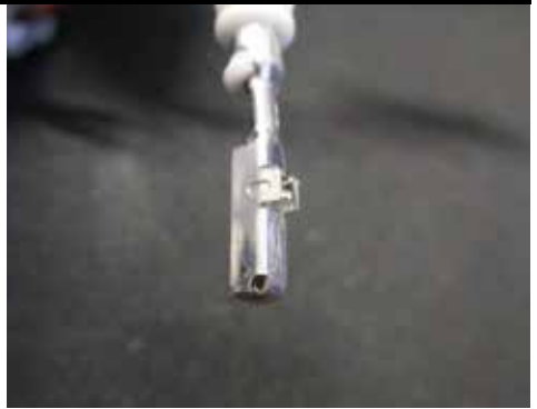
Close up of terminal showing locking tab area
