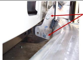
FIT STEEL MOUNT TO REAR OF FUP USE 4  $\frac{1}{2}$ " x  $\frac{5}{8}$ " BOLTS SUPPLIED TIGHTEN ALL BOLTS
