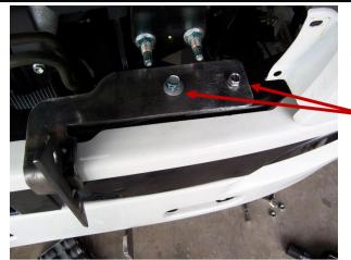
REMOVE GREY SECTION OF GRILL AND REMOVE BOLTS FROM HEADLIGHT FRAMES
