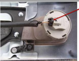
TO EXTEND THE LIGHT CABLE ON DRIVER SIDE BARE INNER CABLE TO SEE WIRE COLOURS AS PER DIAGRAM
