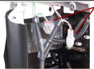
CONNECT WIRING HARNESS SUPPLIED TO BOTH LAMPS THEN CONNECT THE ORIGINAL HARNESS TO THE SUPPLIED HARNESS AS SHOWN
