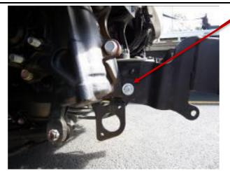
ATTACH MOUNT TO DRIVER SIDE USING ONE (1) 1½" x ½" BOLT AND NYLOC NUT WITH FLAT WASHERS
