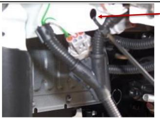
CABLE TIE HARNESS TO HOLE IN BODY SO PLUGS DO NOT HANG LOW AS SHOWN IN PHOTO
