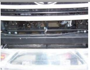
USE CABLE TIES TO SECURE HARNESS TO MOUNT
