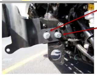
ATTACH MOUNT TO PASSENGER SIDE FRONT HOLE USING ONE (1) 1½" X ½" BOLT AND NYLOC NUT WITH FLAT WASHERS
