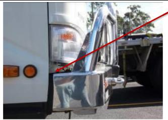
TIGHTEN FRONT EYEBOLTS AND ALIGN THE BULLBAR PARALLEL TO FRONT OF CABIN AND CHECK HEIGHT AT EITHER SIDE
