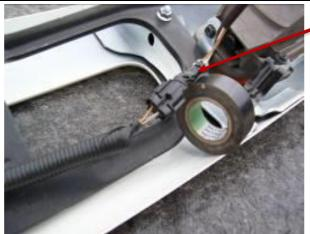
WRAP NEW HARNESS WITH INSULATION TAPE AND CONTINUE UP TO PLUG
