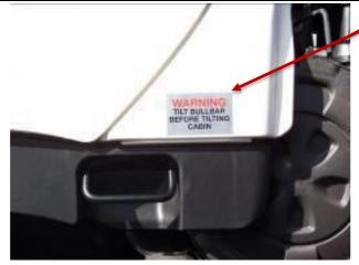
PLACE WARNING LABEL ON PASSENGER SIDE NEAR CAB LIFTING HANDLE AS SHOWN
