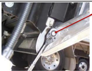
LOCATE PIVOT POINTS AND FIT TWO (2)  $2\frac{1}{2}$ " x  $\frac{9}{16}$ " BOLTS, TWO (2) NYLOC NUTS AND FOUR (4) FLAT WASHERS
