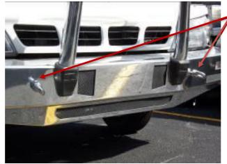
ATTACH BULLBAR TO MOUNT USING TWO (2) EYEBOLTS AND WASHERS PREVIOUSLY REMOVED
