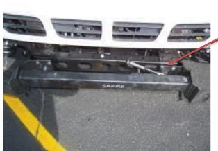
REMOVE STEEL MOUNTING BRAKCET FROM BULLBAR
