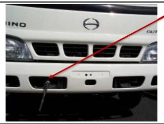
REMOVE FRONT BUMPER BY REMOVING THE 6 8mm BOLTS IN THE FRONT AIR VENT HOLES
