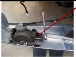
LOCATE ADJUSTING ARM WITH 16mm X 6mm BOLT, WASHER AND WHIX NUT
