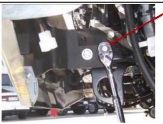
TIGHTEN SIDE BOLTS OF MOUNTS
