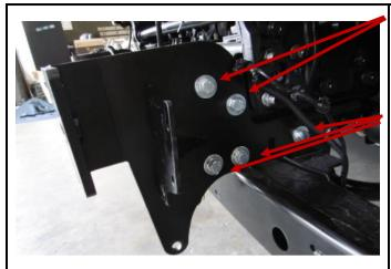
PLACE CHASSIS MOUNT IN POSITION AND FASTEN LIGHTLY THROUGH THE CHASSIS HOLES NOT FITTED WITH CAPTIVE NUTS USING ½" x 2" BOLTS, FLAT WASHERS AND NYLOC NUTS
