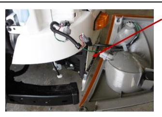
OPEN BONNET AND REMOVE INDICATOR FASTENERS
