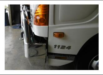
ALIGN THE BULLBAR WITH THE VEHICLE AND TIGHTEN ALL CHASSIS MOUNT FASTENERS FULLY
