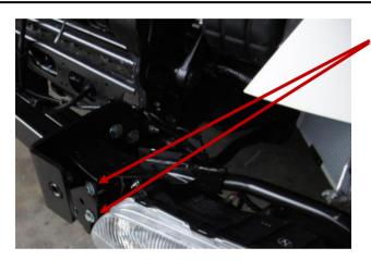
FASTEN HEADLIGHTS LIGHTLY ONTO THE CHASSIS MOUNT EACH SIDE USING 8 - 3" x 3/8" BOLTS, FLAT WASHERS AND NYLOC NUTS
