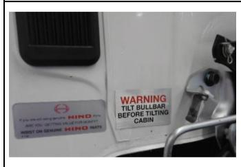
FIT TILT BULLBAR WARNING STICKER TO PASSENGER SIDE REAR OF CABIN NEAR TILT LEAVER
