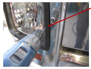
USE A 1/8" DRILL BIT TO DRILL A HOLE INTO THE BULLBAR
