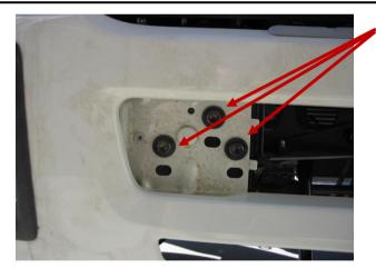
REMOVE BUMPER BOLTS, THREE (3) PER SIDE
