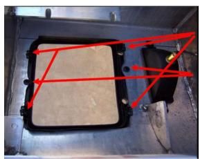
INSTALL HEADLAMP SURROUND INTO BULLBAR USING ORIGINAL FOUR (4) CLIPS
