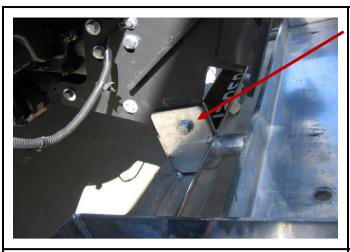
FIT BULLBAR ONTO MOUNT USING TWO (2) 2 X 5/8" BOLTS, WASHERS AND NYLOC NUT
