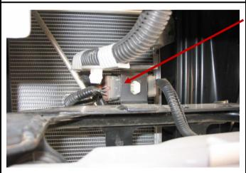
UNPLUG HEADLAMP WIRING FROM CONNECTOR AND HEADLAMP MOUNTING BRACKET
