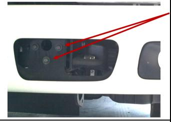
REMOVE TWO (2) OUTER BUMPER RETAINING BOLTS FROM FRONT OF BUMPER ON BOTH DRIVER AND PASSENGER SIDE
