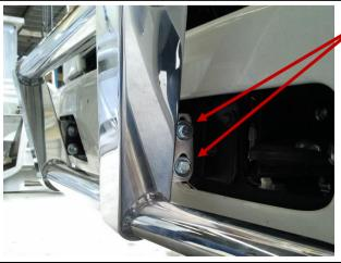
FIT NUDGE BAR TO OUTSIDE OF MOUNTS AND SECURE USING 1 1/4" x 3/8" BOLTS, FLAT WASHERS, SPRING WASHERS AND NUTS
