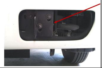
FIT MOUNT BRACKETS TO VEHICLE USING ORIGINAL BOLTS
